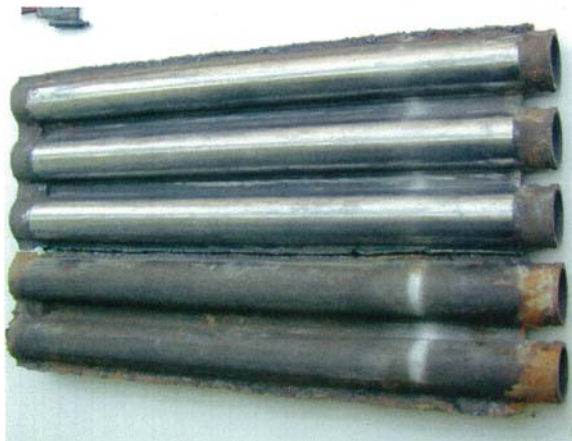
Fig. 8 Appearance of furnace wall tubes after 24 months of service
